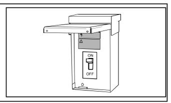
**STEP 4** - Wait one (1) hour before starting the unit if compressor crankcase heater is used and the outdoor ambient temperature is below 70 °F.
