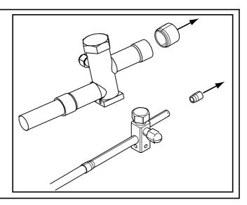
**STEP 2** - Remove the pressure port cap from both service valves.
