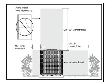
Position unit to allow adequate space for unobstructed airflow, wiring, refrigerant lines, and serviceability.
